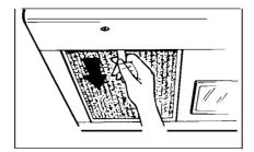
**To remove grease filter,** grasp the "finger hold" on the filter and slide to the rear.
